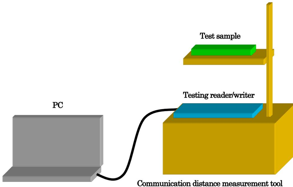
Figure 5-3 Equipment Configuration for the Interoperability Test
