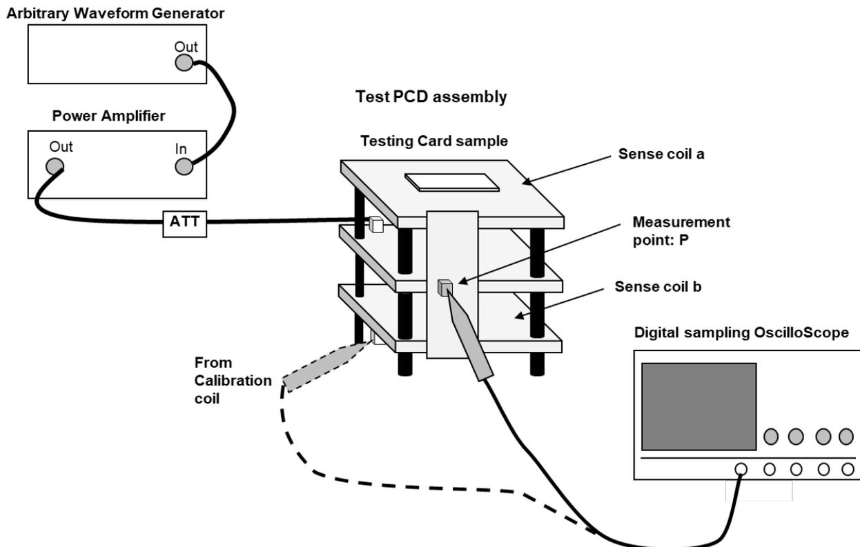
Figure 5-2 Example configuration of equipment for basic performance testing<sup>51</sup>
