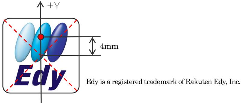
Figure 6-2 Measurement Center Point of the Eddy Touch Operation Terminal
